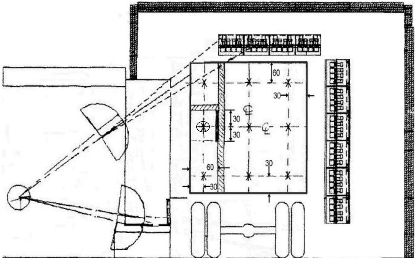
**Source and collimator assembly and shield**
